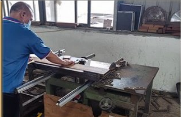
6,Precision cutting of WPC profiles according to requirements
