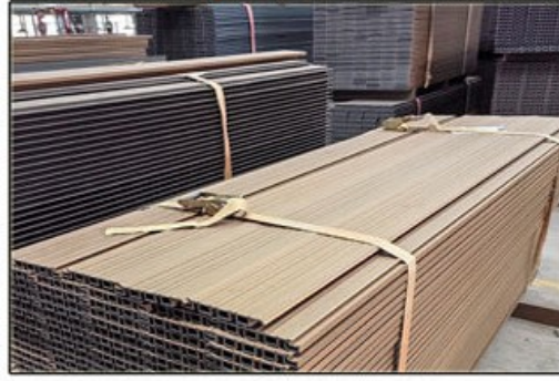
4,The extruded profiles must be neatly bundled and cooled.
