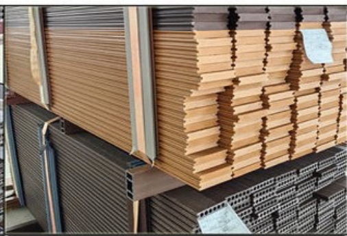
4,The extruded profiles must be neatly bundled and cooled.
