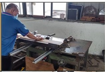
6, Precision cutting of WPC profiles according to requirements
