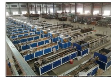
3, The extruder extrudes the raw material into profiles using a mold
