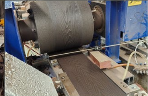
3,The extruder extrudes the raw material into profiles using a mold
